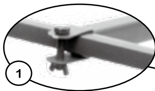
FIGURE 7 ADJUSTABLE SUPPORT BAR ASSEMBLY INSTALLED (LADDER SHOWN UPRIGHT FOR CLARITY)
