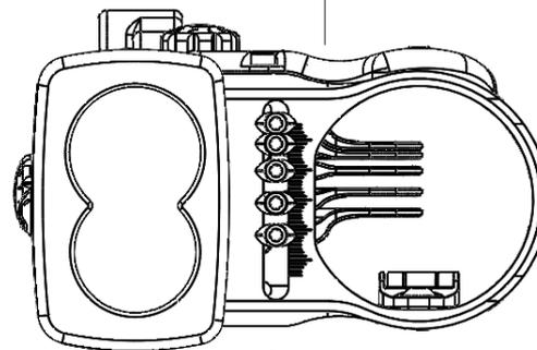
\*Pins can be removed if archer prefers more open optics by completely removing the machine screw on the preferred pin and gently removing the pin housing from the bezel.
