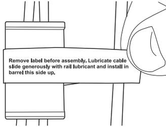
Remove protective label from cable slide before crossbow assembly
