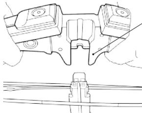
Assemble bow unit onto tip of barrel after cable slide and bowstring are properly positioned
