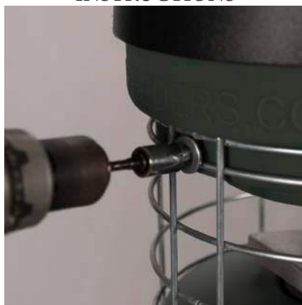
Step 11: Bolt powerhead to cage using (3) SM Washers and (3) Bolts.
