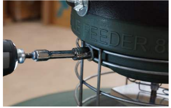
Step 10: Bolt powerhead down. (3) SM Washer (3) Bolt
