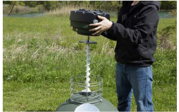
Step 10: Place powerhead on top of cage.
