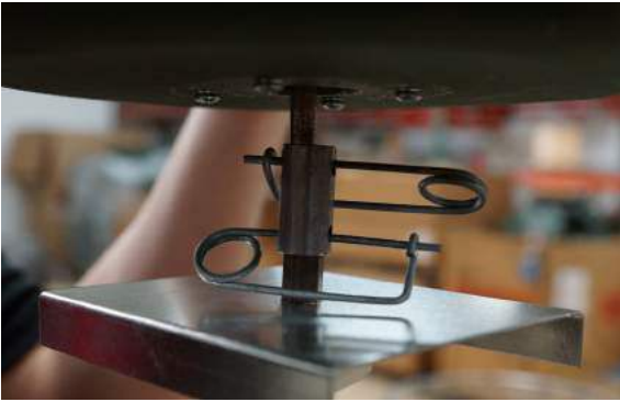
Step 9: Attach 1 end coupler to motor at- tach other end to auger. Insert safety pins.
