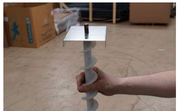
Step 8: Place spinner on top of auger.
