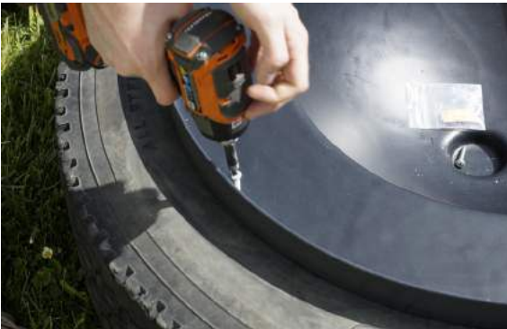
Step 3: Attach base to tire. (4) Tire screws
