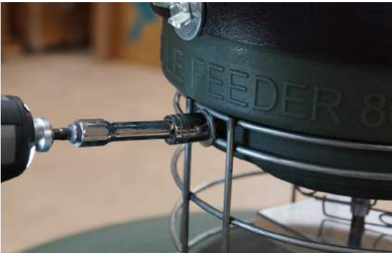
Step 11: Bolt powerhead down.
