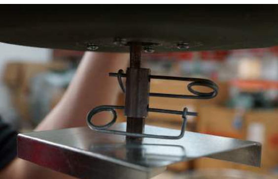
Step 7: Attach 1 end coupler to motor at- tach other end to auger. Insert safety pins.
