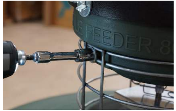
Step 10: Bolt powerhead down.
