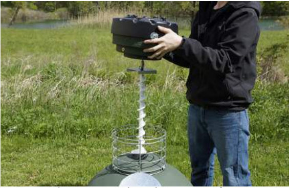
Step 9: Place powerhead on top of cage.
