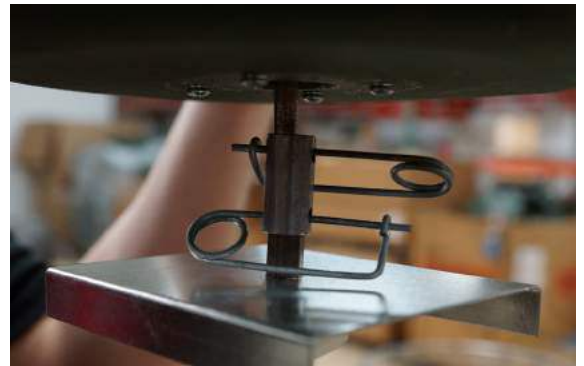
Step 12: Attach 1 end coupler to motor attach other end to auger. Insert safety pins.
