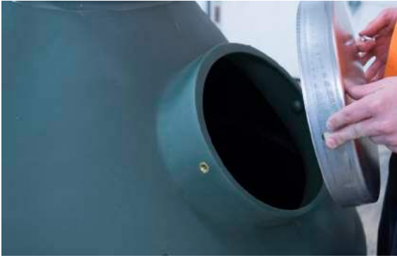
Step 9: Attach fill cap (2) Wing Nut
