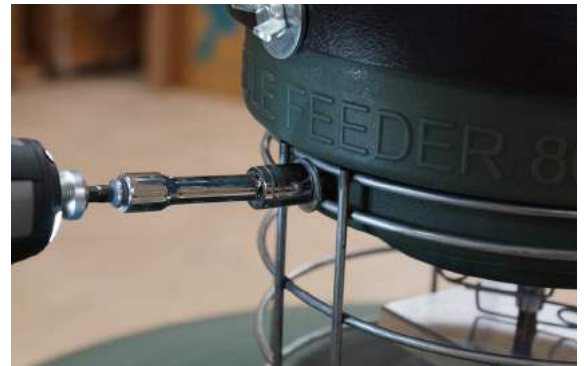
Step 14: Bolt powerhead down. (3) SM Washer (3) Bolt
