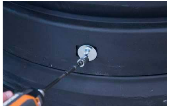
Step 4: Attach extension ring to base.
